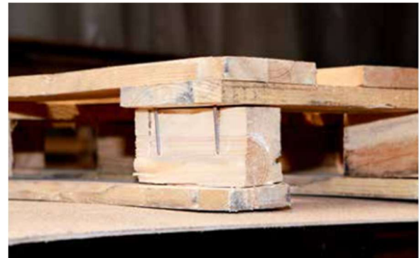
Visible fasteners e.g. nails
