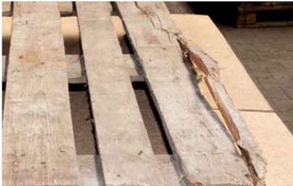
Diagonally, transversally or partially broken board
