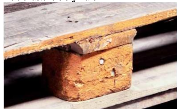
Contamination e.g. paint, oil, mould
